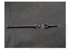
These are the parts you will need to assemble the cvd. Part names from left to right. CVD shaft, 5mm barrel, M2x12mm pin, CVD axle and 1/2" spiral retaining ring. The spiral retaining ring keeps the pin from coming out. This is our preferred method. However we did include some set screws, to lock down the pin through the barrel (if using this method it is best to grind a small flat on the pin, to keep the pin from walking out. Also use Loctitie on set screw).
