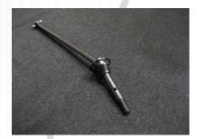
This is the cvd fully assembled. Simply slide the cvd axle into the bearing carrier and you are ready to go.
