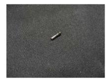
You will need to save the set screw pin, from the stock half shafts.
