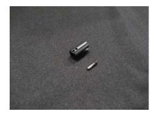
The set screw pin will be used to attach the drive cup to the diff shaft. (Note: the cup has 2 holes, these are for different shock positions.) Use the hole that will give you the most suspension travel.
