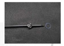
With all the cvds parts installed, it is now time to slide the spiral retaining ring over the cvd axle and onto the groove to capture the pin. (Note: I have used shrink tubing over the assembly to seal out dirt, however this is an option.)
